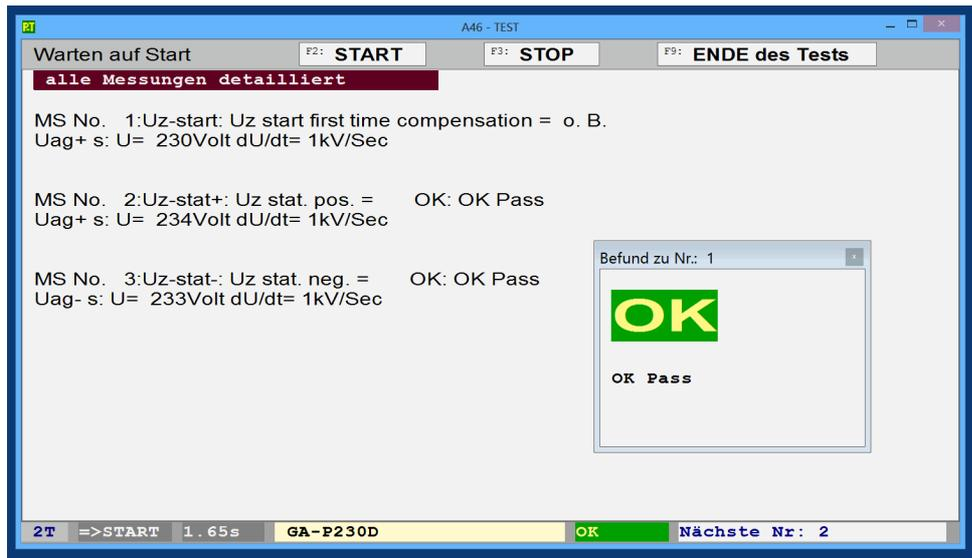
Detailed list of measured values, results and position of all measurements
