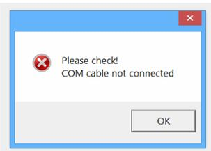
A working interface is found but no COM-cable. May be the COM-cable is connected to another interface.
